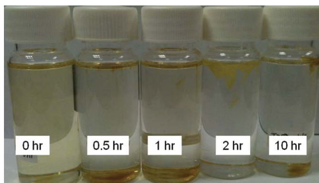
Figure 14. Solubility tests in solvent NMP of the CD-grafted PAI asymmetric membranes modified with m-XDA-β-CD for varied times.
